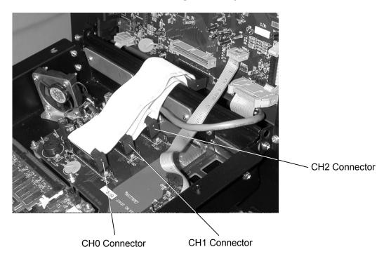
Figure 9-3 Channel Connections in Type A FCO
